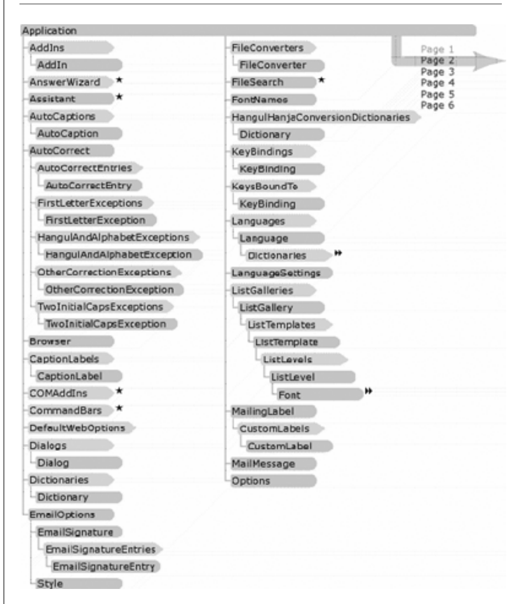
FIGURE 2 Extension of the Word Document Model Showing More of the Tree and Leaf Object Structure
